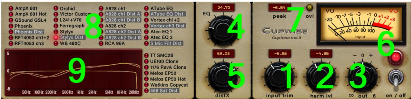
1. **Input Trim** – This input gain control has output compensation which keeps your output level constant so you only hear the tonal changes while boosting or lowering the input.
